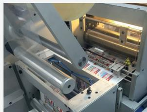
Unwind for self-adhesive unsupported laminates. Fast and trouble free protection of digital print. Optional support paper rewind.
