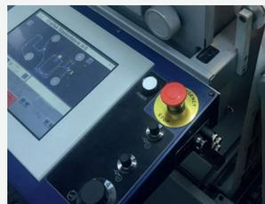
Large 10" color touch display with clear indication of web path. Knobs for stepless tension setting on rewind spindels.
