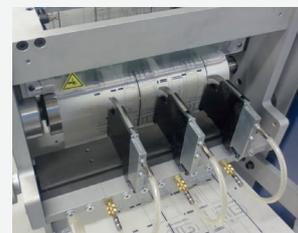
Pneumatic crush knives with fast set screw. Knives are controlled from touch screen. Set your slitting up in a few minutes.
