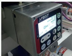
As standard the unit features a BST web guide with an ultra sonic fork. The web guide supports normal and transparent webs.
