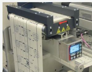
Splice table with tape dispenser and airclamps for easy and break-free splicing.
