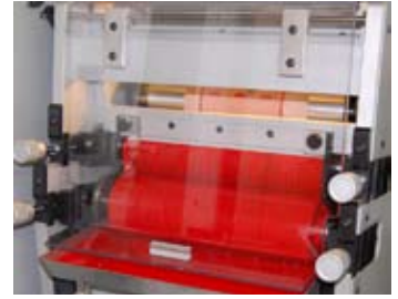
The flexographic printing station can run as a full flood varnish station or a spot varnish in register to pre-printed web.
